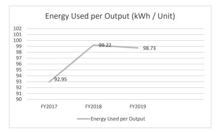
Notwithstanding the fact that cylinders output in FY2019 was 360 cylinders lower than in FY2018, however, energy used per output was lower due to the scrapping of 5 machines. The 5 machines were previously on standby mode to minimise repair and maintenance costs while new machines are being phased in.
